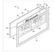
The inventors of the present application developed novel optically active materials, methods, and articles. One embodiment of the present application is an optically active article, comprising: an infrared-reflecting material positioned adjacent to an optically active substrate such that the infrared-reflecting material forms a pattern that can be read by an infrared sensor when the optically active substrate is illuminated by an infrared light source.
