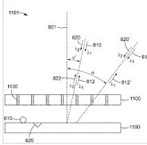
A retroreflective system is disclosed that includes a retroreflective sheet for retroreflecting light, and a light control film disposed on the retroreflective sheet. For a first wavelength, light incident on the light control film at each of a first and second angles of incidence is retroreflected. For a second wavelength, light incident on the light control film at the first, but not the second, angle of "incidence is retroreflected.
